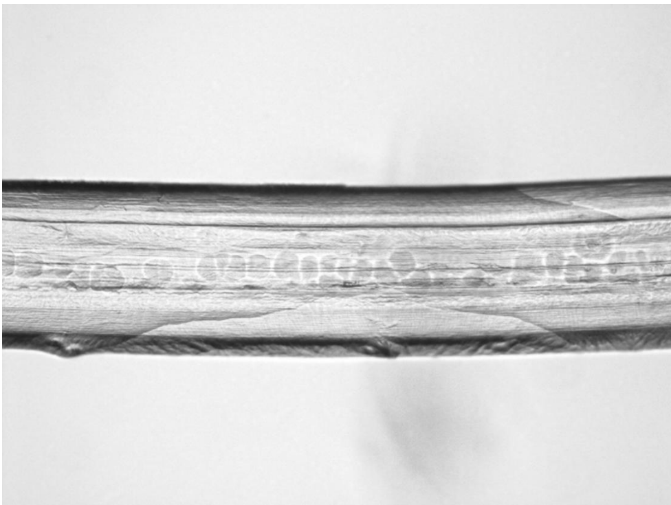
Micrograph of a printed fibre with encapsulated cells.
